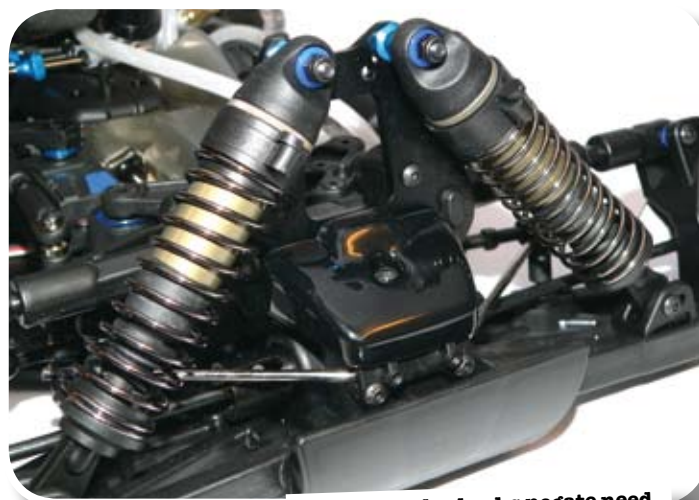
Raked angle shocks negate need for large, exposed shock tower
